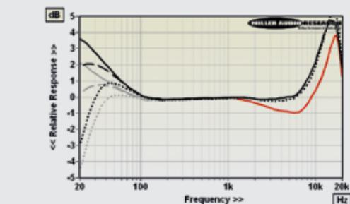
**ABOVE:** Freq. resp. (-8dB re. 5cm/sec) lateral (L+R, black) vs. vertical (L-R, red) vs. stereo (dashed). Bass only: Output 1/30Hz, solid; 2, dashed; 3, dotted; Output 1/50Hz, grey solid; 2, dotted; 3 dashed)
