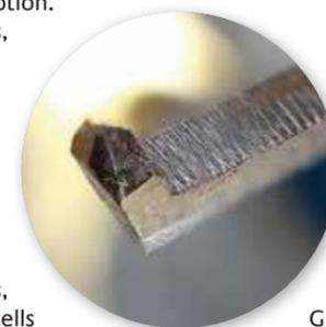
**LEFT:** Micrograph reveals the laser-trimmed diamond cantilever with right-angled tip cut into a 'Micro-Ridge' profile
