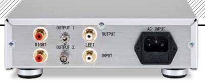
**ABOVE:** Rear view of the DS-E1 PSU/equaliser. The pick-up's internal LED is powered via the R- and L- pins while the output is returned via R+ and L+, all via the 'Input' RCAs. The equalised outs are also on RCAs (Output 2 with a deeper subsonic filter)
