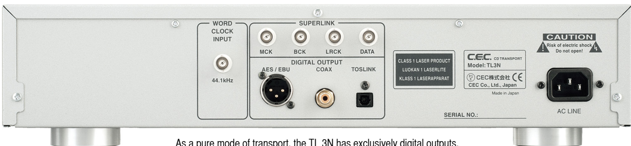
As a pure mode of transport, the TL 3N has exclusively digital outputs.
