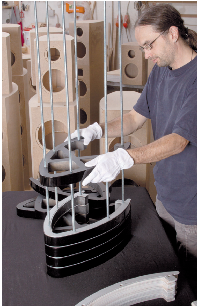
First the ribs are loosely stacked. The pressure necessary for stability is provided by the bars.
